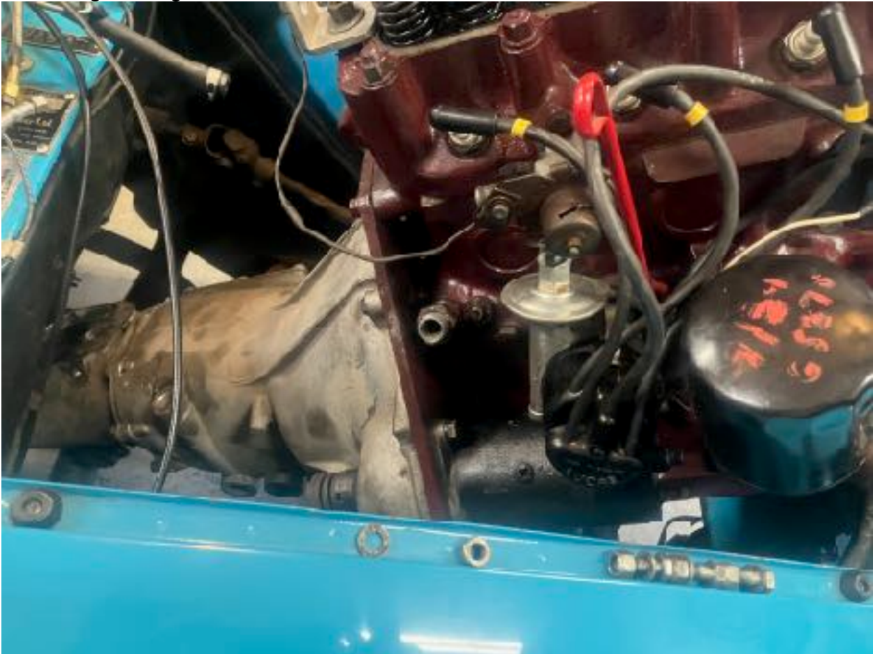
Removing the engine and transmission from an MGA
